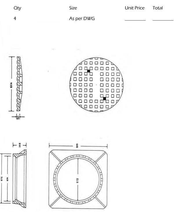
2. High impact HDPE flat manhole grade adjustment rings.
