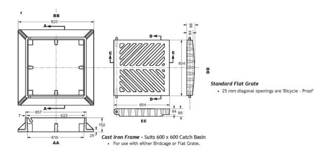
2. The Town of Labrador City requires the supply of sewer manhole covers and Frames as per the attached diagram.
