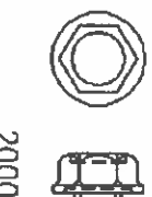
200001945 NUT LOCK HEX NYLON INSERTED M10 x 1.5
