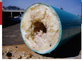
**Grease Filled Pipe** Help Prevent Sewer Blockages By
