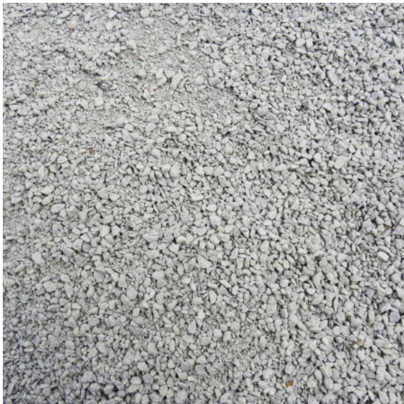
Crusher Dust Hiking Trail Surfacing
